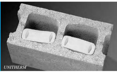
**Composition and Materials: UNITHERM** Inserts are individually molded from expandable polystyrene in a minimum density of 1.3 lbs. per cu. ft. Inserts are packaged at the point of manufacture in heat-sealed, clear polyethylene bags.
